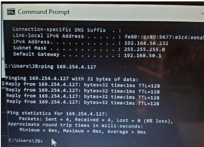
Figure A-42. Ethernet Connection Using Once Device.
