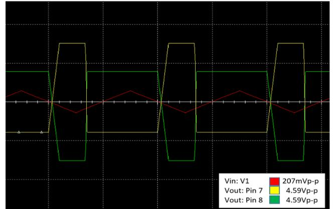
Figure A-23. LT1713 Simulation Results with triangular input wave.
