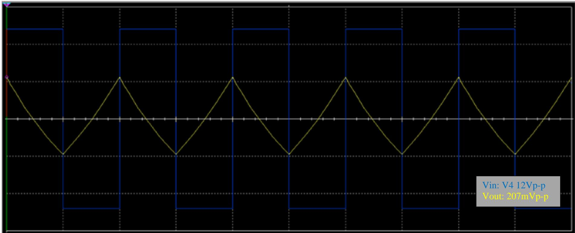
Figure A-20. OPA694 Simulation Results using an input pulse wave.
