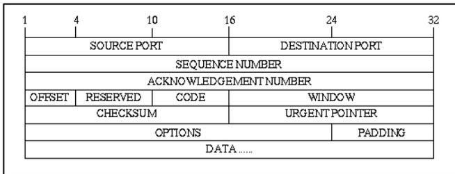
Figure A-9. TCP Segment Header Format. [25]
