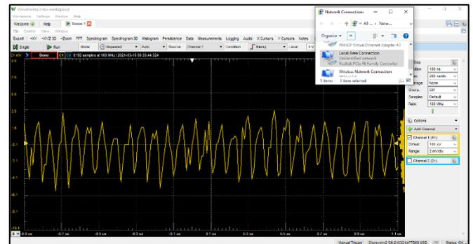
Figure A-31. The encoded signal at the output of our receiver's current feedback amplifier.
