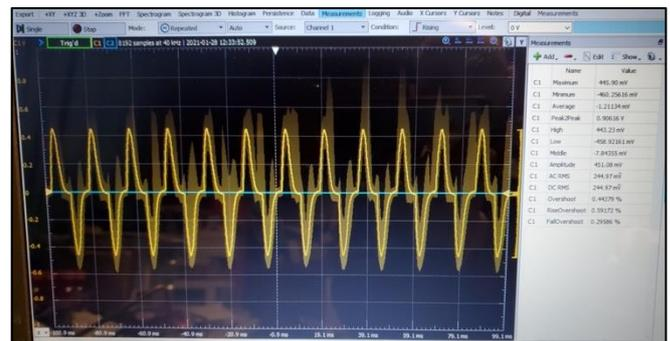
Figure A-29. Ethernet Signal Detection.
