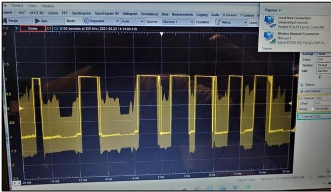
Figure A-34. Improved signal at the buffer stage of the receiver.
