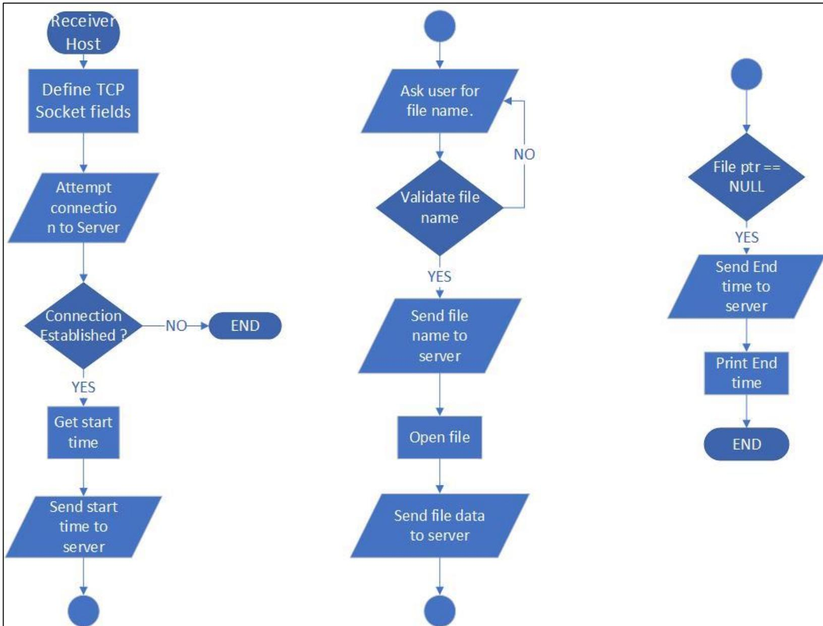
Figure D- 2. Client Socket Flowchart
