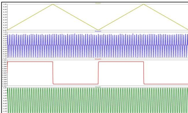
Figure A-26. Simulation Results from MAX4392.
