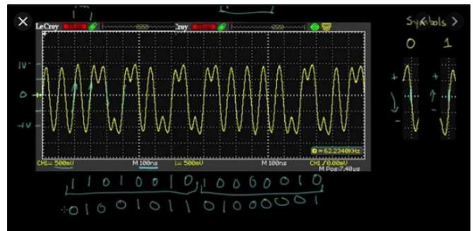
Figure A-30. Theoretical representation of ethernet signal using Manchester's encoding scheme. This image was captured from one of Ben Eaters YouTube videos. Check out his channel for all sorts of cool stuff. [129]
