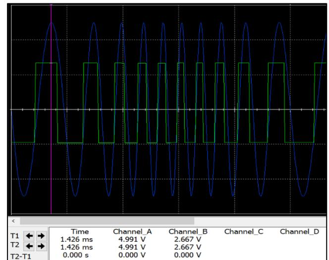
Figure A-24. FM Input Signal LT1713 Simulation Results.
