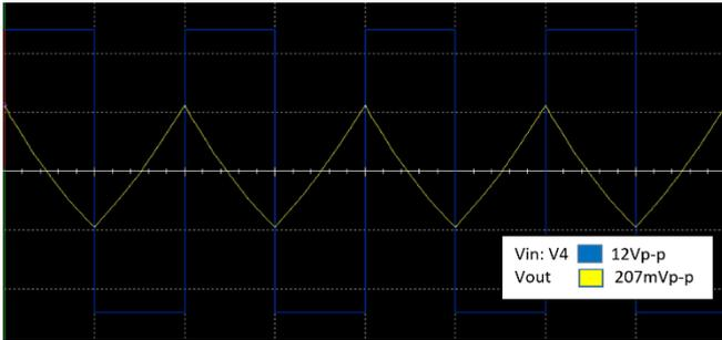
Figure A-20. OPA694 Simulation Results using an input pulse wave.
